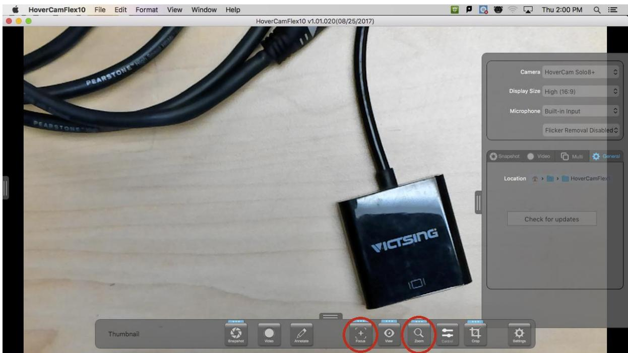
Focus and Zoom buttons as well as additional functions are accessed via the HoverCam tool bar.
